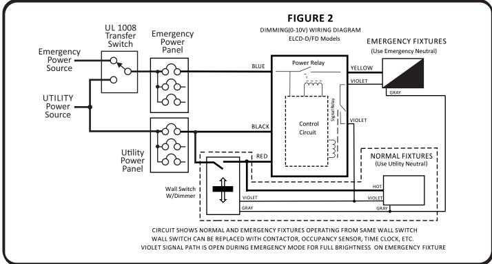
Figure 1 and Figure 2 illustrate typical wiring for Non-Dimmed and Dimmed Loads
