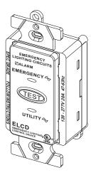
IMPORTANT – The ELCD does not transfer two nonsynchronous power sources. Emergency Power is continuously fed from the lighting inverter and provides the source of power for emergency fixtures under all modes of operation. Utility Power is only a sense line which causes a relay closure between the Emergency Power's Input/Output.
